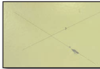
Galvanite™ cold rolled sheet steel with our powder coat finish after a 336 hour salt spray test.
